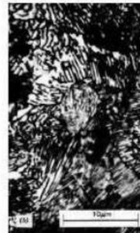
Figure: Microstructure resulting from Different Cooling Rates Applied to Austenitized Samples of Eutectoid Steel
