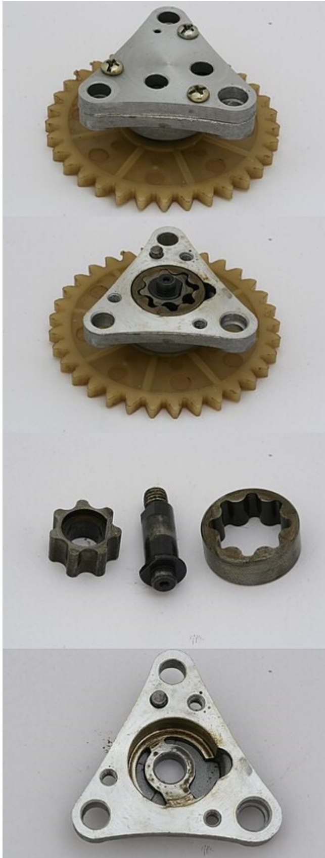
As the gears rotate they separate on the intake
