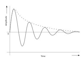
Fig. 7.4. Damped vibrations
