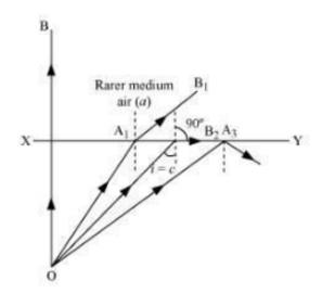
Fig. 8.3 Total internal reflection
