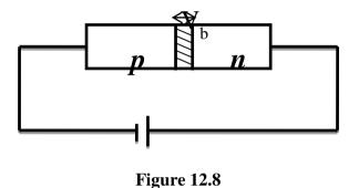
The external voltage pulls the majority carriers holes in the p-type crystal and the electrons in the n-type crystal away from the junction. This increases the width of depletion layer. The diode offers very high resistance and no current is set up across the Junction due to majority carriers. However a small current may be there across the junction due to minority carriers. It is called leakage *current* ( $I_s$ ).
