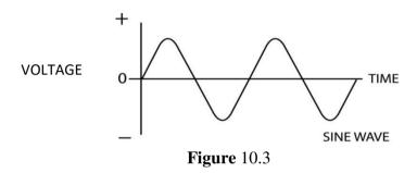
The radio frequency current in antennas and transmission lines are the examples of AC.
