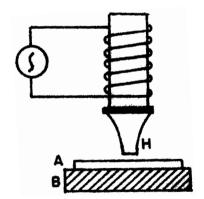
Fig. 7.7 Ultrasonic drilling
