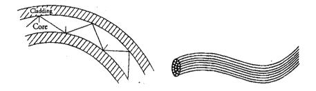
Figure 13.4 Schematic of optical fibre
