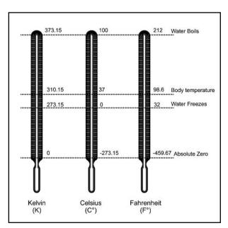
taken as zero Kelvin (-273° C). At absolute zero temperature, the pressure (or volume) of the gas goes to zero. This may implies that if the temperature is reduced below -273.15°C, the
