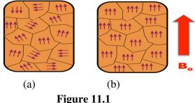
These domains are usually randomly oriented as shown in Fig. 11.1 (a) and net magnetism is zero in the absence of magnetic field. When an external field is applied, the domains reorient themselves to reinforce the external field as shown in Fig. 11.1 (b) and produce a strong internal magnetic field that is along the external field.
