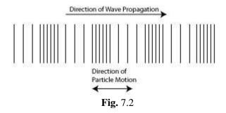
Most familiar example of longitudinal waves is sound waves. Sound waves can travel in medium such as solids, liquids and gases.
