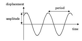
Fig. 7.5. Undamped vibrations
