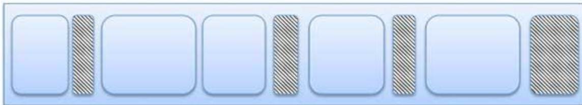
Fragmented memory before compaction
