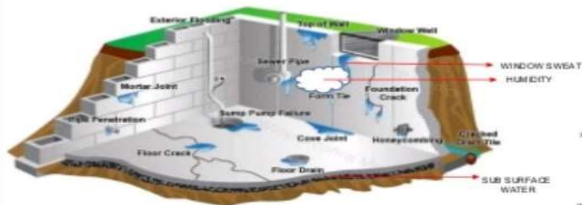
DIAGRAM SHOWING THE DIFFERENT TYPE OF LIQUID LEAKAGE/ SEEPAGES IN BASEMENTS
