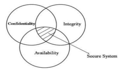
The diagram above explains the balance concept. The right balance of the three goals is needed to build a secure system. If the goals are not balanced then a small hole is created for attackers to nullify the other objectives of security. Having a highly confidential system but low availability then the system is not secure.
